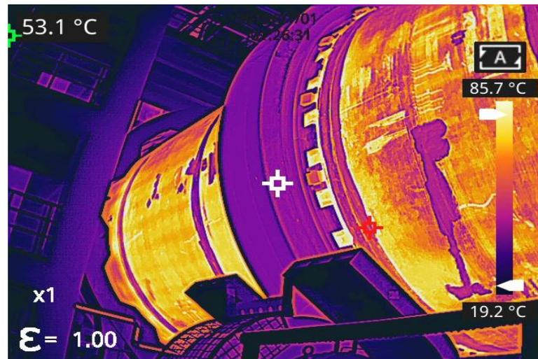
Rotary Kiln Defect Monitoring
