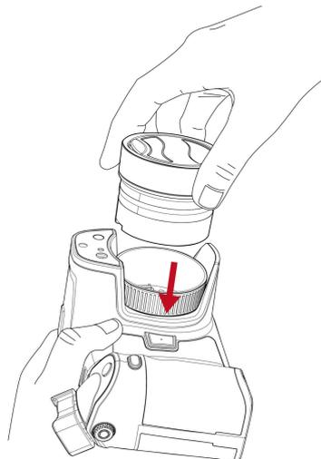
6. Rotate the lens 90° clockwise. The lens makes a click when it locks in place.
