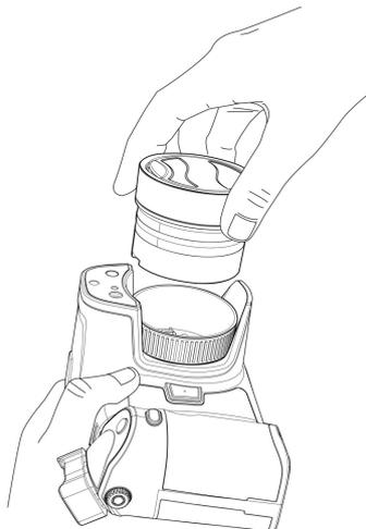
3. The infrared detector is now fully exposed. Do not touch this surface. If you see dust
