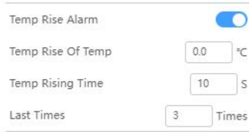
Figure 3.8 Measurement List-Temperature Rise Alarm Settings
